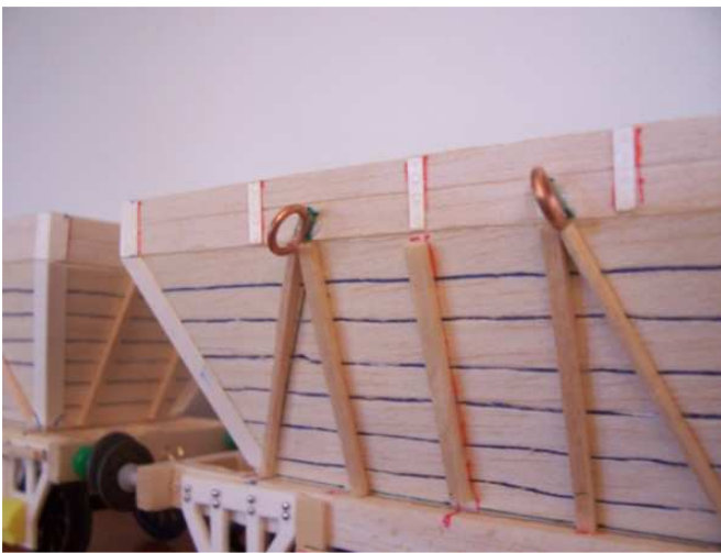
1.6mm Copper wire circles for Lift Rings.
