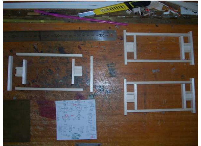
Buffer beams and Sole Bars are cut, glued & squared.
