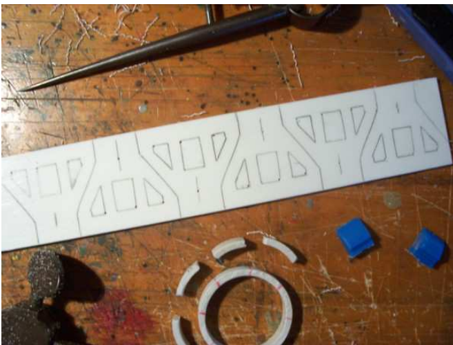
"W" Irons marked on 2mm styrene, brake blocks from 32mm diameter PVC pipe, fret work in progress.
