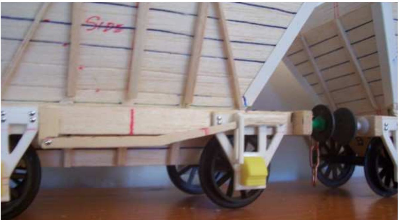
Brake Lever and Keeper Bracket. Couplings are \frac{1}{4} " hooks and fabricated copper 'oval' link chain.
